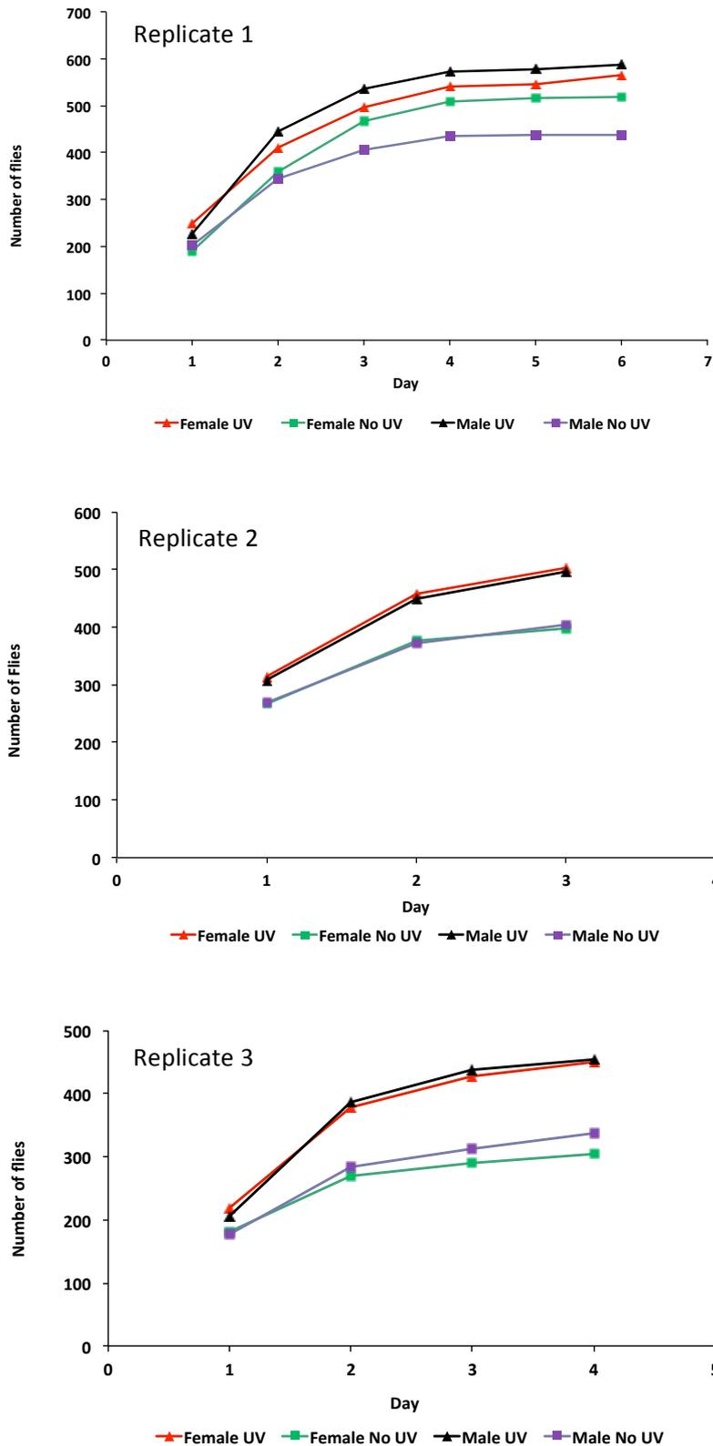
**Figure 8.** Cumulative number of male and female Q-flies killed after landing on toxicant-treated citrus plants that were or were not illuminated by a UV light in a glasshouse setting. Total numbers of captured flies analysed in Table 9 are those reported on the final day of collection in this figure.
