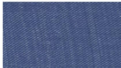
**GroShield** Spunbonded polypropylene 'fleece' used primarily for frost protection but also insect exclusion and reduction of evaporation. Inexpensive but single use only as tears easily. Cohesive barrier (no holes), shading approximately 10-15%, range of thickness/weights from 18-50g/m<sup>2</sup>. Supplied by NetPro Pty Ltd.
