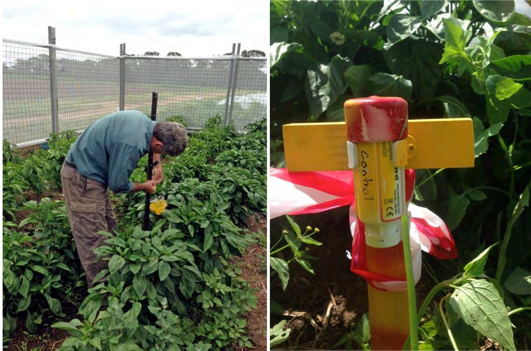
Figure 4 - Installing a fruit fly trap inside a fenced area (L) and a data logger mounted underneath the floating row cover (R)
