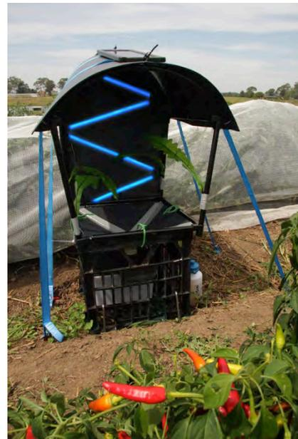
**Figure 5. Prototype UV light trap installed in the chilli crop.**
