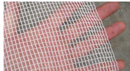
**VegeNet** Knitted white high density polyethylene net designed to exclude larger pests and provide some protection from wind and rain. Mesh size approx. 1 x 3mm, shading 10%, weight 45g/m<sup>2</sup>. Supplied by NetPro Pty Ltd.
