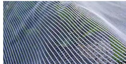
**Aphid Net** Translucent woven material made from high density polyethylene. Designed to exclude most insects and last 8-10 years. Mesh size 0.6 x 0.6mm, shading 14%, weight 45g/m<sup>2</sup>. Supplied by Crop Solutions UK.
