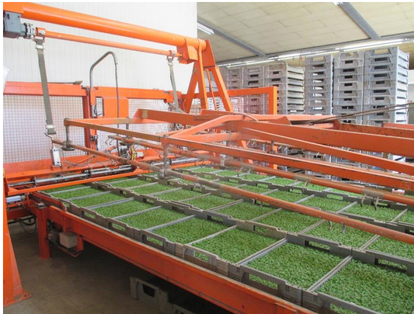
Automation makes it easy to stack and transport seedling trays at Rudolf Sinn GmbH.
