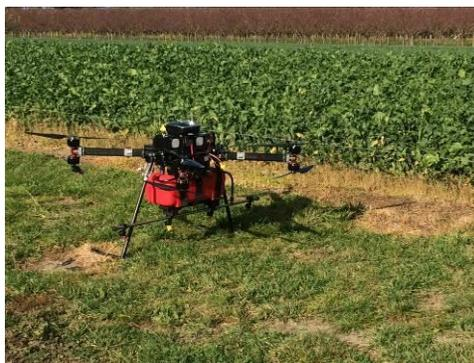
**Figure 12: UAV with 20l spray tank**
