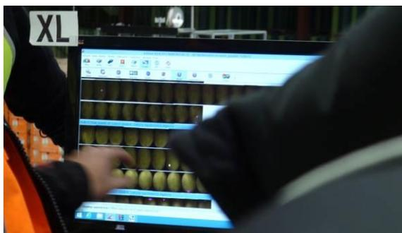
**Figure 9: Grading system software showing NIR images/scans of individual pieces of fruit passing through the grader.**
