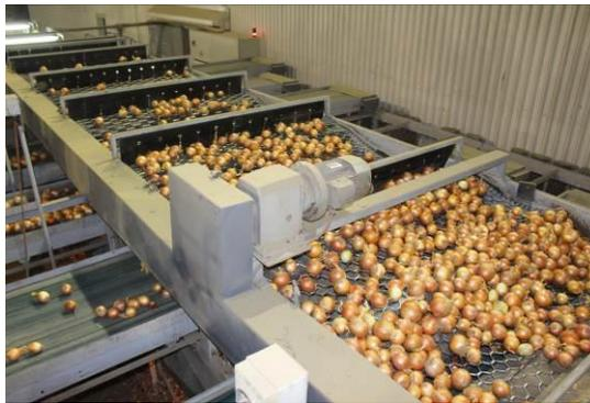
**Figure 19: Onions being graded into sizes**
