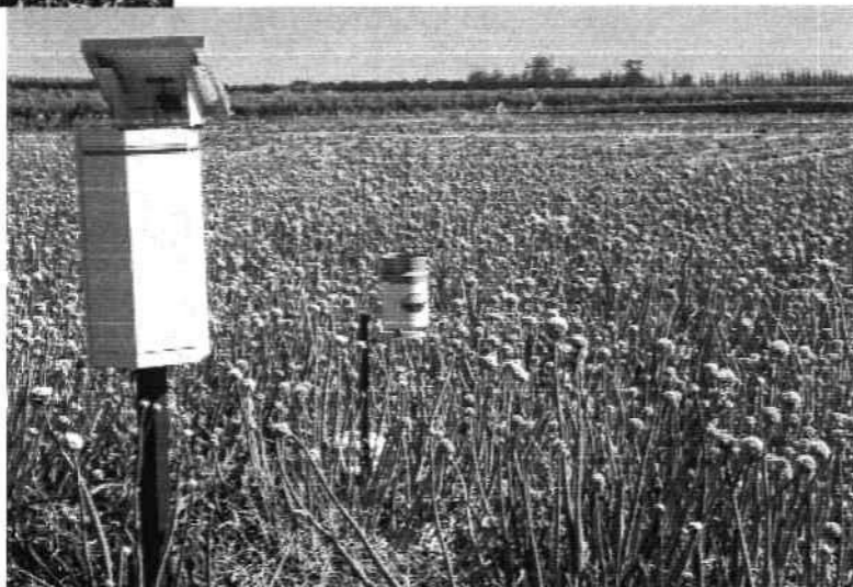
Figure 2 Downy mildew was predicted by a weather-based model on the EnviroCaster unit that was purchased for this project
