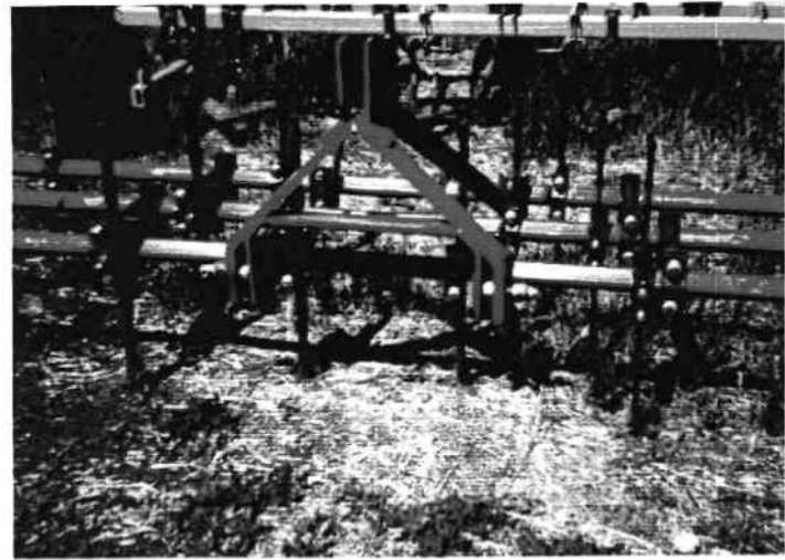
(d). 'Go-Devil' chisels and disc bed-formers
