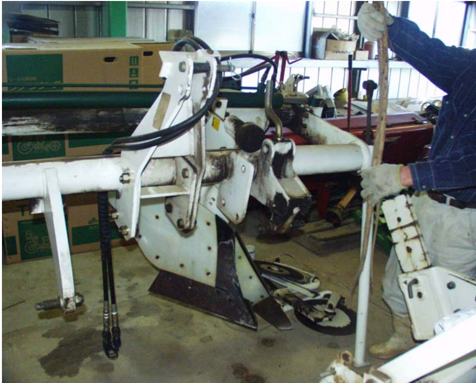
Figure 1: Sugano plough lifter used to harvest burdock roots
