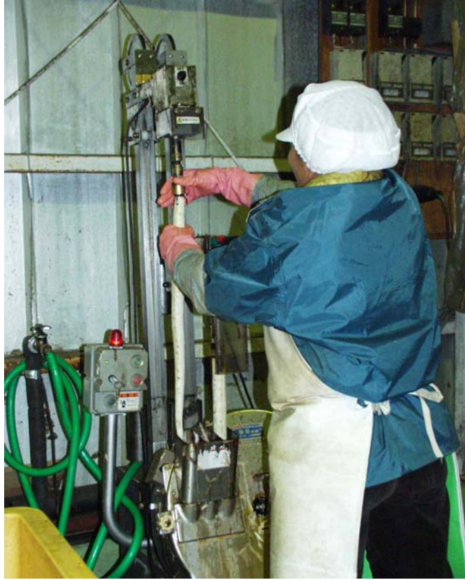
Figure 19: Sasagaki cutter machine
