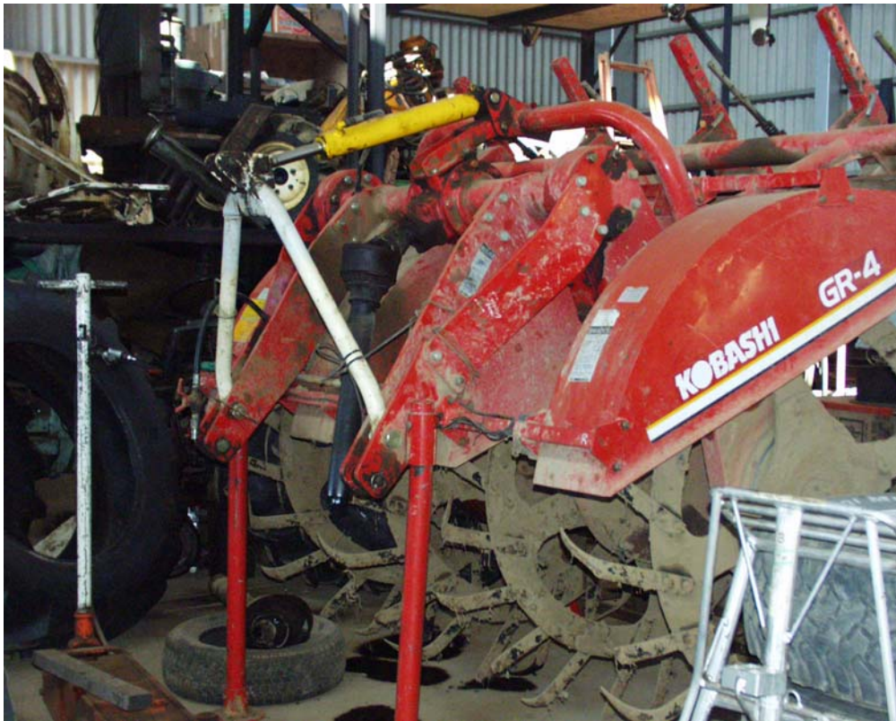
Figure 3: Rotary trencher used to cultivate soil for burdock planting
