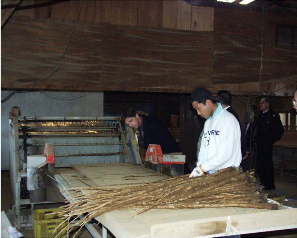
Figure 7: Cutting the stalk off the burdock root using a circular saw.
