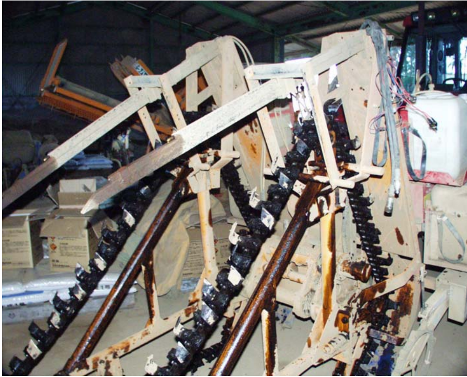
Figure 11: Trencher fixed with probes that applying soil fumigant deep into the soil whilst trenching
