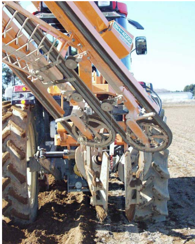
Figure 5: The belts used to lift the burdock root by the crown out of the ground
