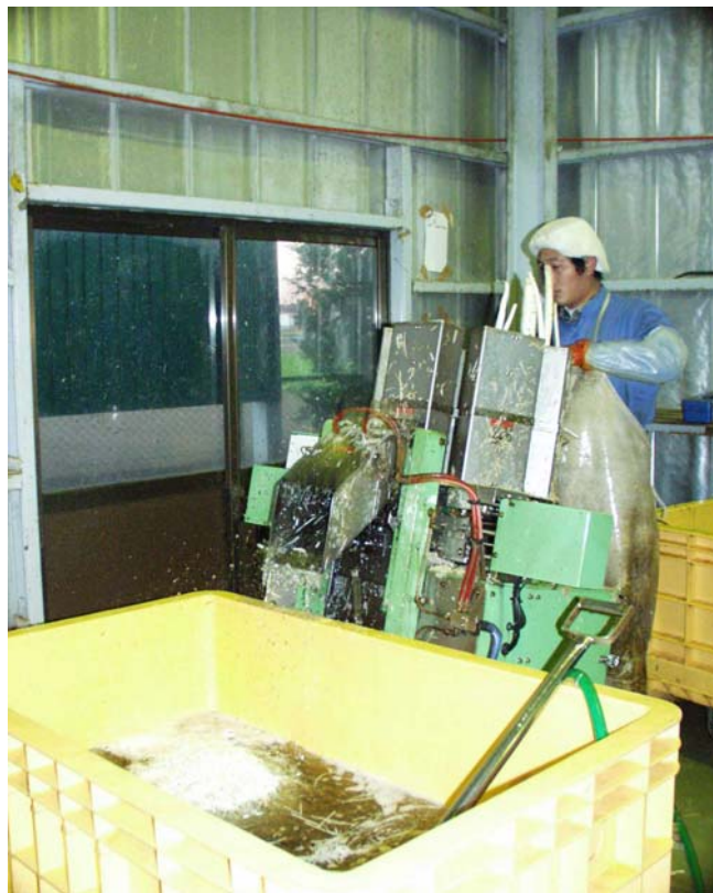
Figure 18: Kimpira cutter machine
