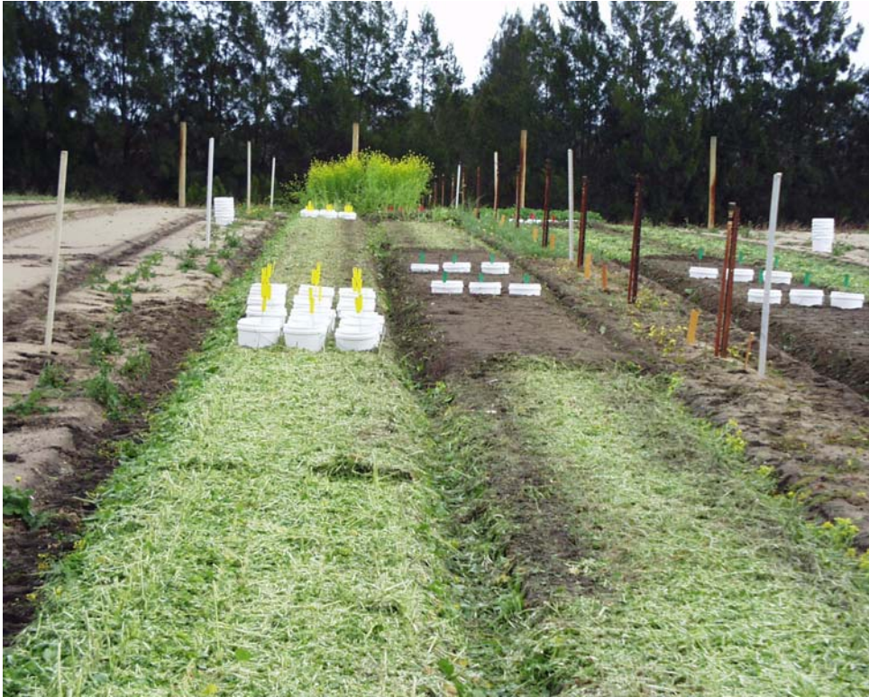
Cylinders for simulated irrigation in different treatments. Intensity of work varies in different plots (most sampling was in Fumus mulched and left on the surface).
