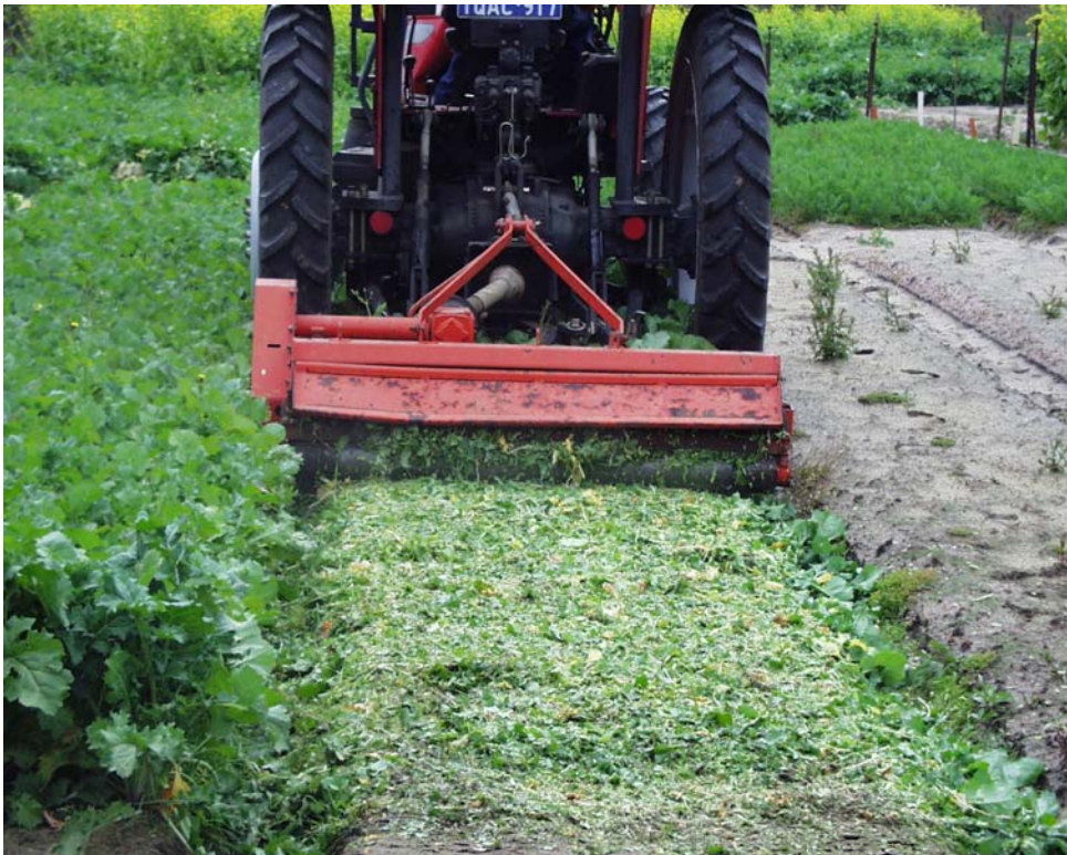
Mulching BQMulch. Note chopped nature of foliage and low velocity of expulsion.
