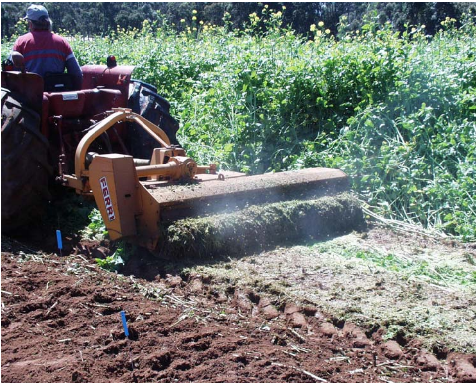
Mulching Fumus mustard. Note spray, which shows extent of pulverisation, and the amount of residue in relation to the initial amount of biomass.
