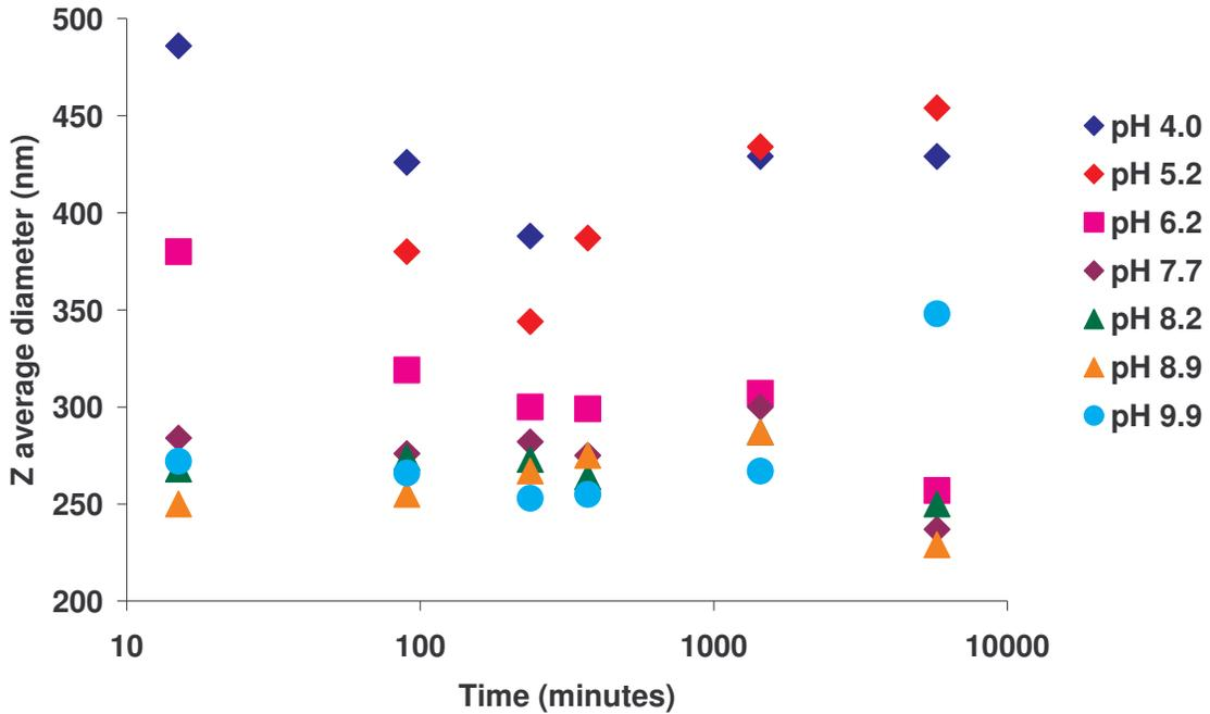
Figure 3: The impact of time and pH on the particle size in a simulated spray tank
