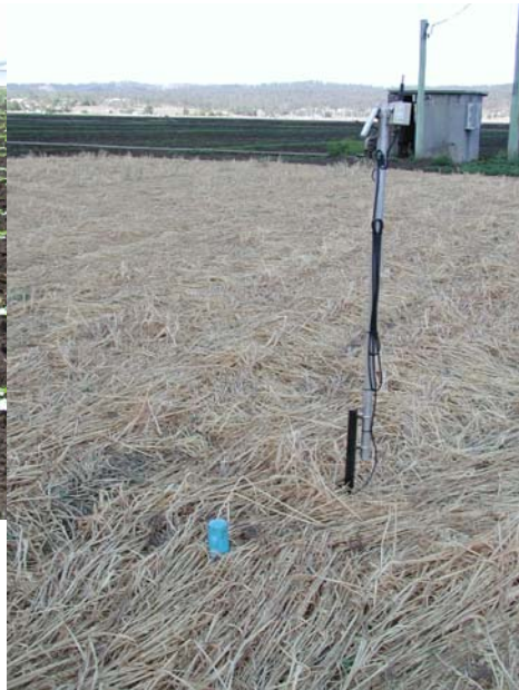
Fig. 23: Soil moisture was logged using a C Probe
