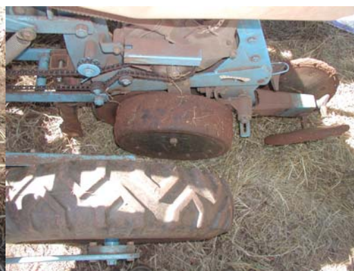
Fig. 87: Rear assembly of planter used for direct seeding vegetable crops into organic mulch
