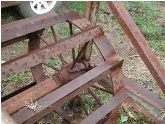
Fig 29: The crimping roller used to flatten the cover crop of millet
