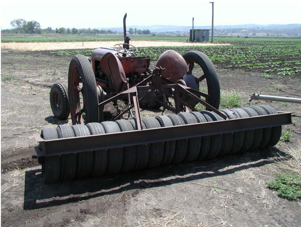
Fig 28: The implement used for rolling the cover crop, after it was killed with herbicide
