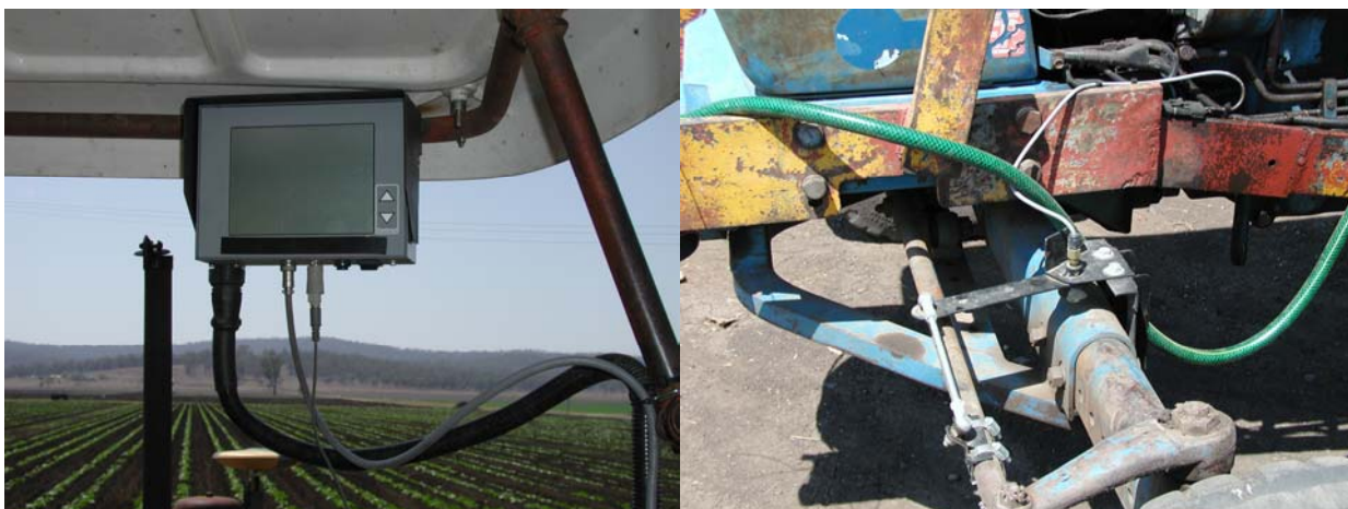
Fig 24 & 25: GPS equipment fitted to tractor cab and steering assembly (right) that can assist in bed formation and planting in a permanent bed system
