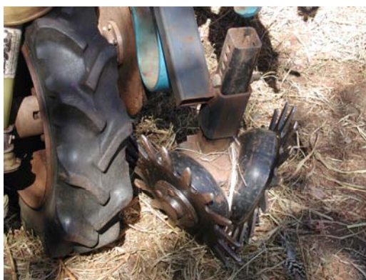
Fig. 86: Forward assembly of planter.
