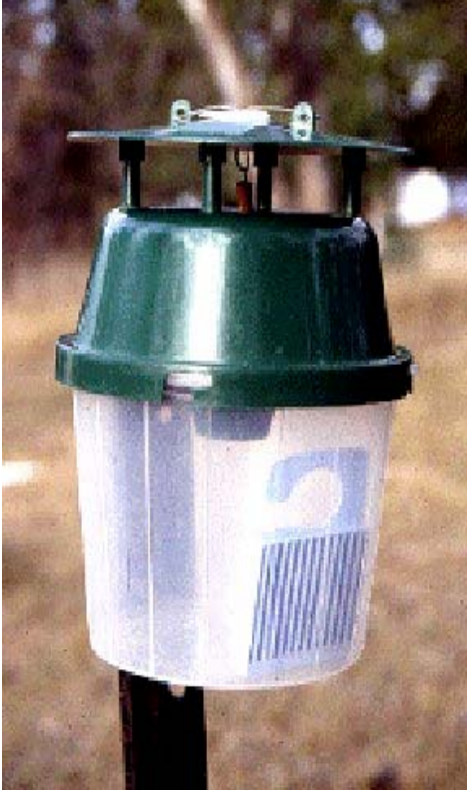
Figure 13 Agrisense pheromone funnel trap. Unlike this trap the traps used in this trial had an opaque green plastic base.
