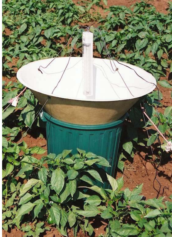
Figure 14 Light trap in capsicum. The full setup used in monitoring also has a 30W solar panel.
