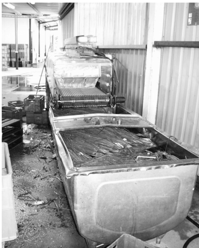
Figure 11 The washing plant used in the experiments. Vegetables were placed on the conveyor where they were pressure washed with fresh water. At the end of the conveyor, vegetables fell into a tank of sanitised water. For the experiments there were two tanks, one containing calcium hypochlorite and the other iodine.
