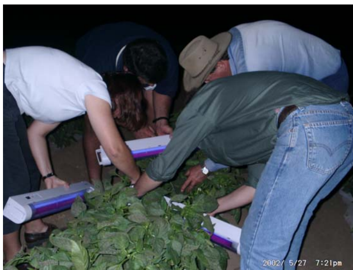
Plate 2: Growers assessing spray droplet coverage using black light (Bundaberg workshop, 22 May 2002)
