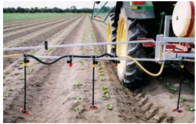
Fitting a conventional boom with droppers and extra nozzles can improve spray coverage.
