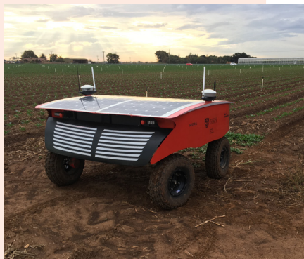
Figure 2: RIPPA demonstrates its ability to autonomously monitor brassica crops in Werribee
