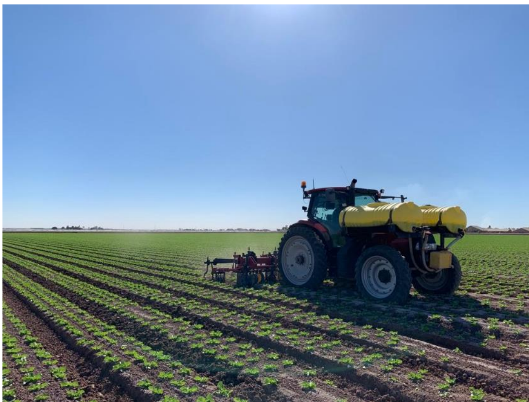
GPS Tractor making 42 inch beds.
