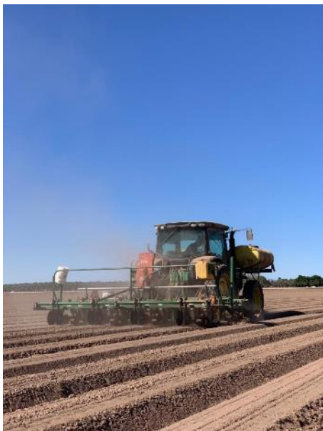
GPS Tractor making 42 inch beds.
