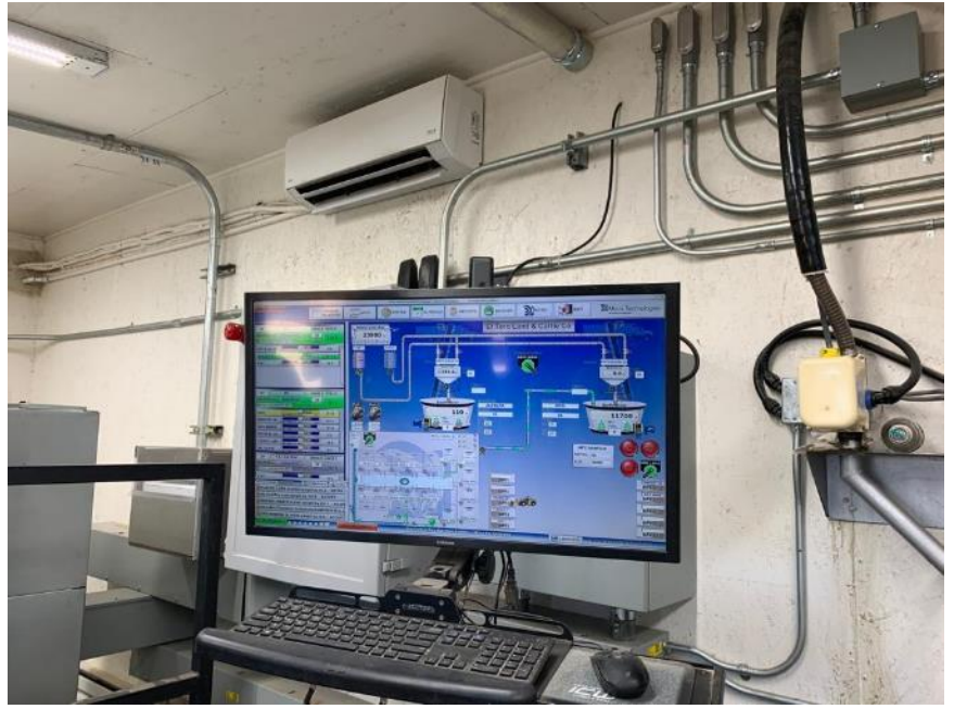
Each tractor has a computer system inside the cab, just like the computer on the right. The computer includes the recipe for the order and the tray of the tractor is weighted to enable the driver to know how much of each ingredient they have collected as well as having the weight of the mixing bin so they can ensure measurements of the tractor are accurate.
