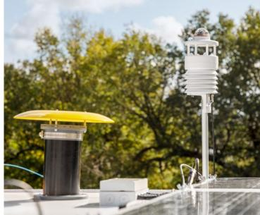
Sentinel trapping devices including the two-metre insect trap, spore sampler, and weather station.
