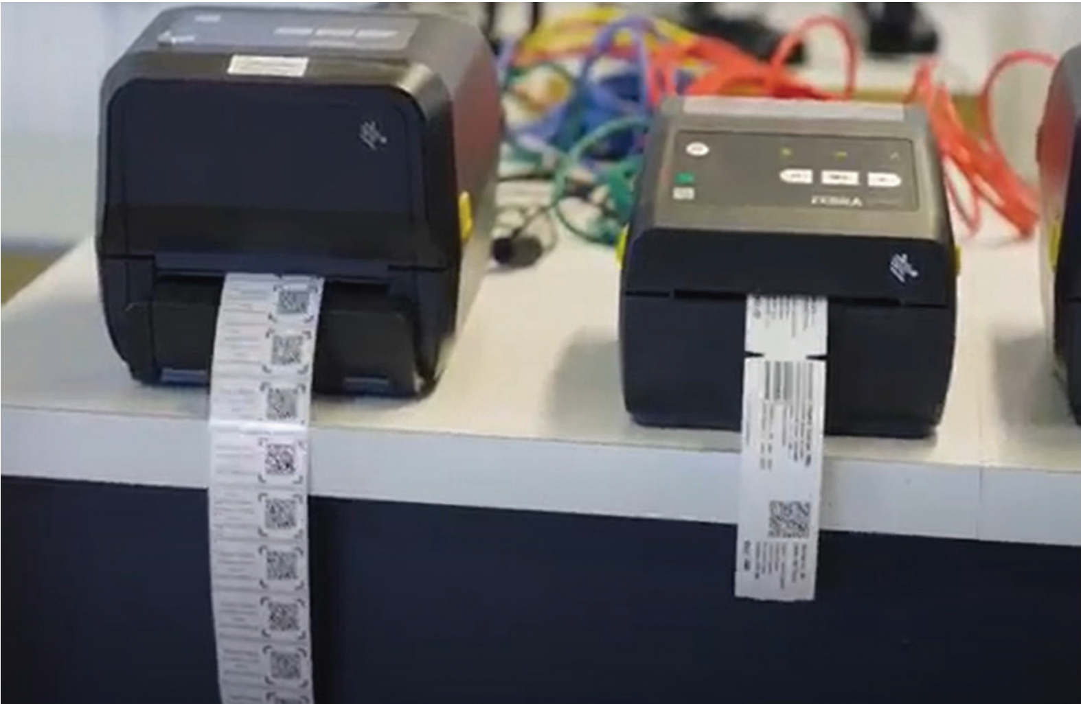
Figure 2. Printing on-demand labels deployed by FreshChain systems in the cherry packhouse.
