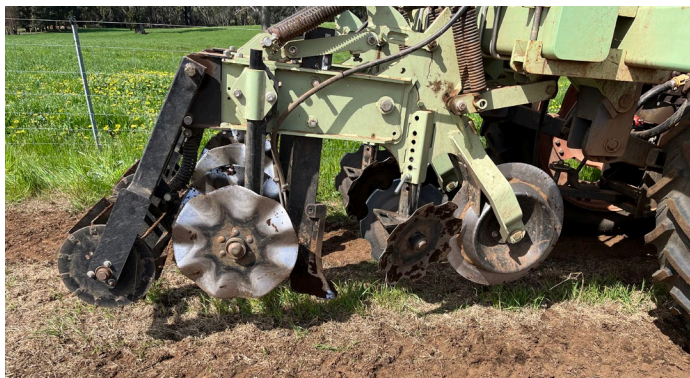
Figure 5: An example of a strip-till machine.
