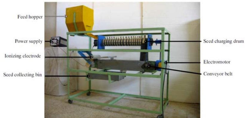
Figure 2. An electrostatic separator used for experimental purposes to separate wheat, canola and barley seeds with high and low germination (Basiry & Esehaghbeygi, 2012).
