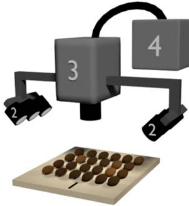
Figure 11. Thermal imaging equipment that was used to collect information about viability of Norway spruce seeds, used to classify seeds as viable, empty or infested with 98-99% accuracy (Dumont et al. , 2015). Numbering shows (1) the seed lot, (2) halogen lamps that pulse light onto the seeds, (3) an infrared camera that captures the thermal images, (4) the control unit that processes the data.
