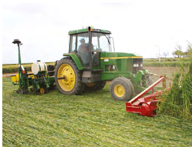
Roller-crimping a ryecorn cover crop and direct seeding in one pass. Photo courtesy of Rodale Institute
