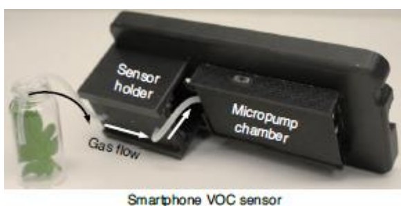
Figure 8: E-nose for detection of disease of plant foliage (Li et al. 2019)
