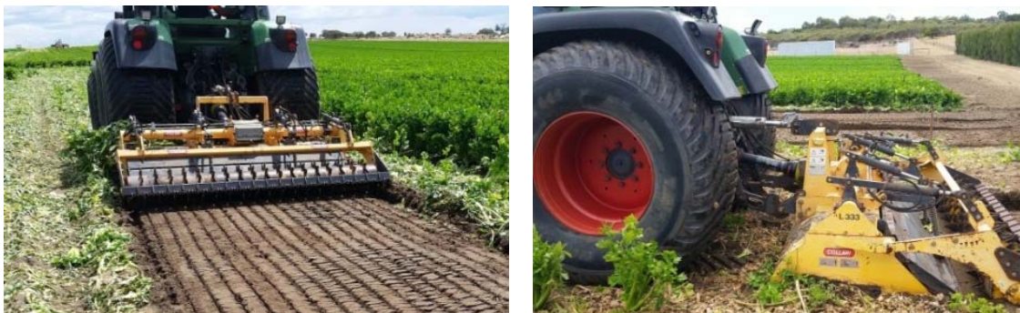
Figure 1. A Collari stone burier going over celery crop residues 1day (LHS) or 7 days (RHS) after harvest
