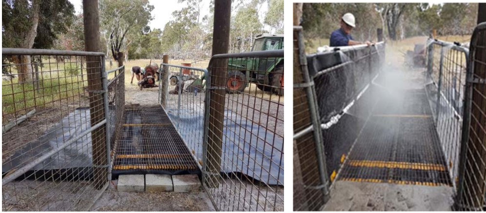
Figure 40. Final construction of the Cattle Walk Through Fly Trap (LHS), with the side jets triggered as cattle walk on through the race (RHS)
