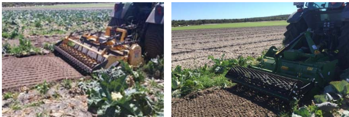
Figure 42. Each stone burier machine burying cauliflower crop residues left after harvest
