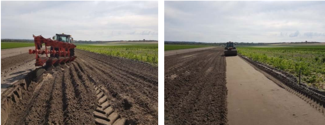
Figure 3. A mould board plough burying celery residues (L) and a land roller compacting the soil (R)
