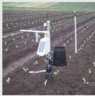
Example of the in field node which is used to capture rainfall and irrigation data, readings of soil moisture in one of the lettuce field trials.
