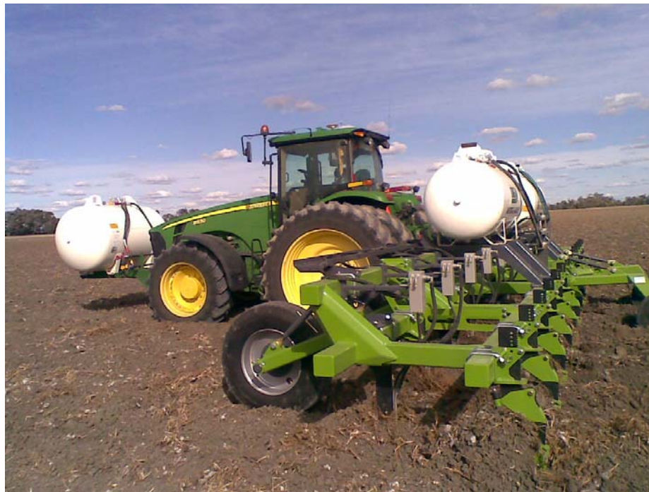
Figure 4. Anhydrous ammonia Big N application equipment using tines. Photo courtesy of Incitec Pivot Fertilisers.
