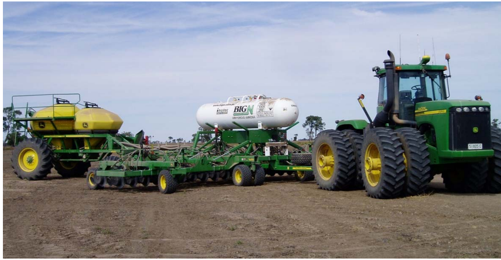
Figure 2. Application equipment using discs. Photo courtesy of Incitec Pivot Fertilisers.
