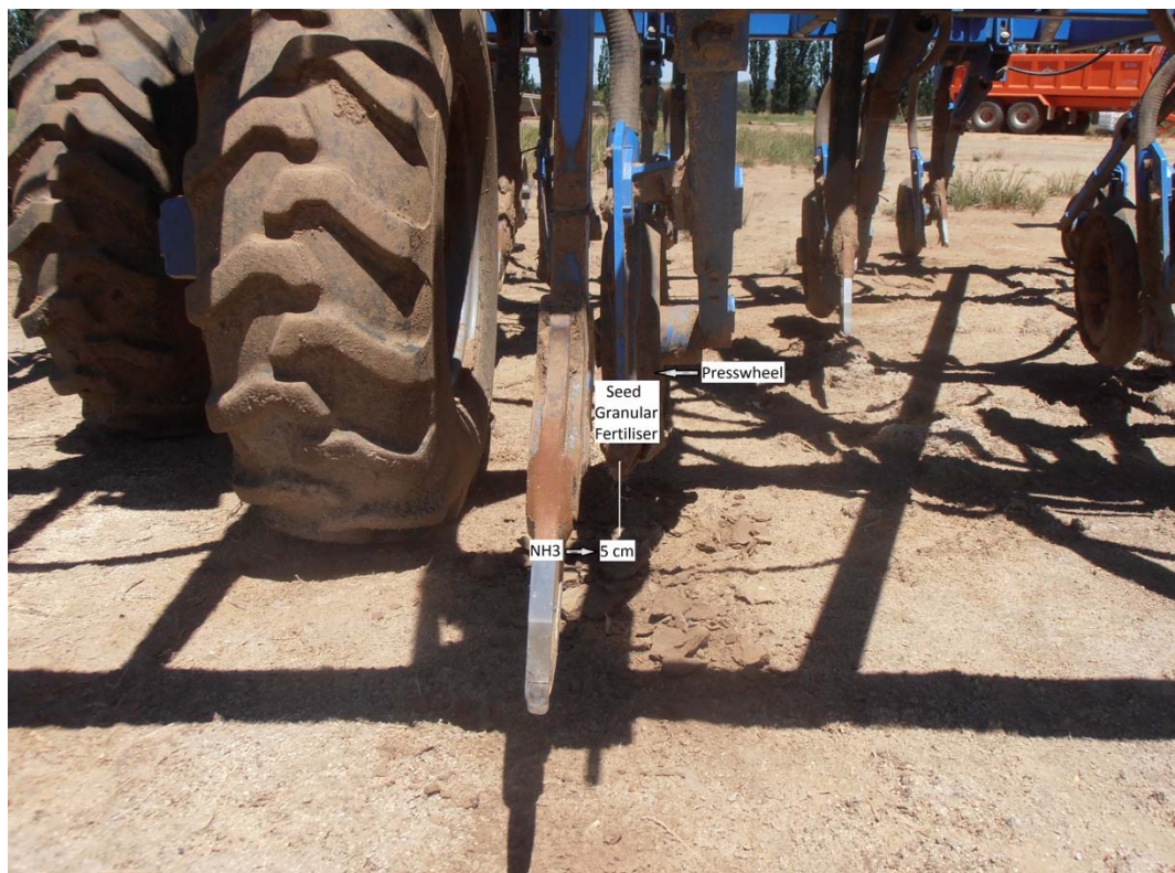
Figure 6. Front view of the knifepoint for anhydrous ammonia and granular seed/ fertiliser on the application equipment on the commercial vegetable farm in Cowra, NSW.
