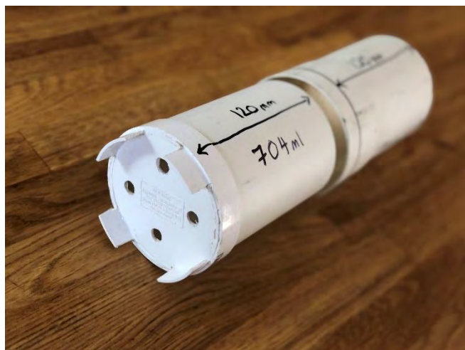
Figure 13. An AFP measuring device is cheap and easy to make and is an invaluable tool for substrate testing.
