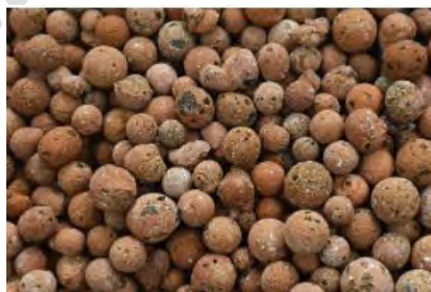
Figure 12. Expanded clay pellets are used in flood and drain and home hydroponics.
