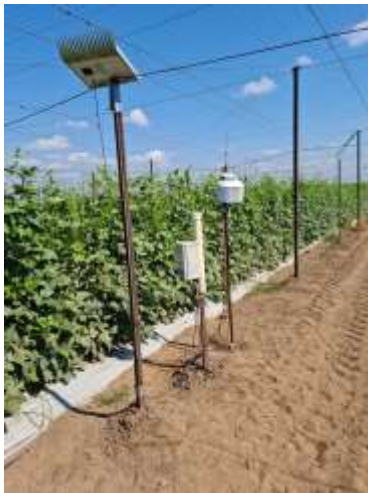
Soil moisture probe on site
