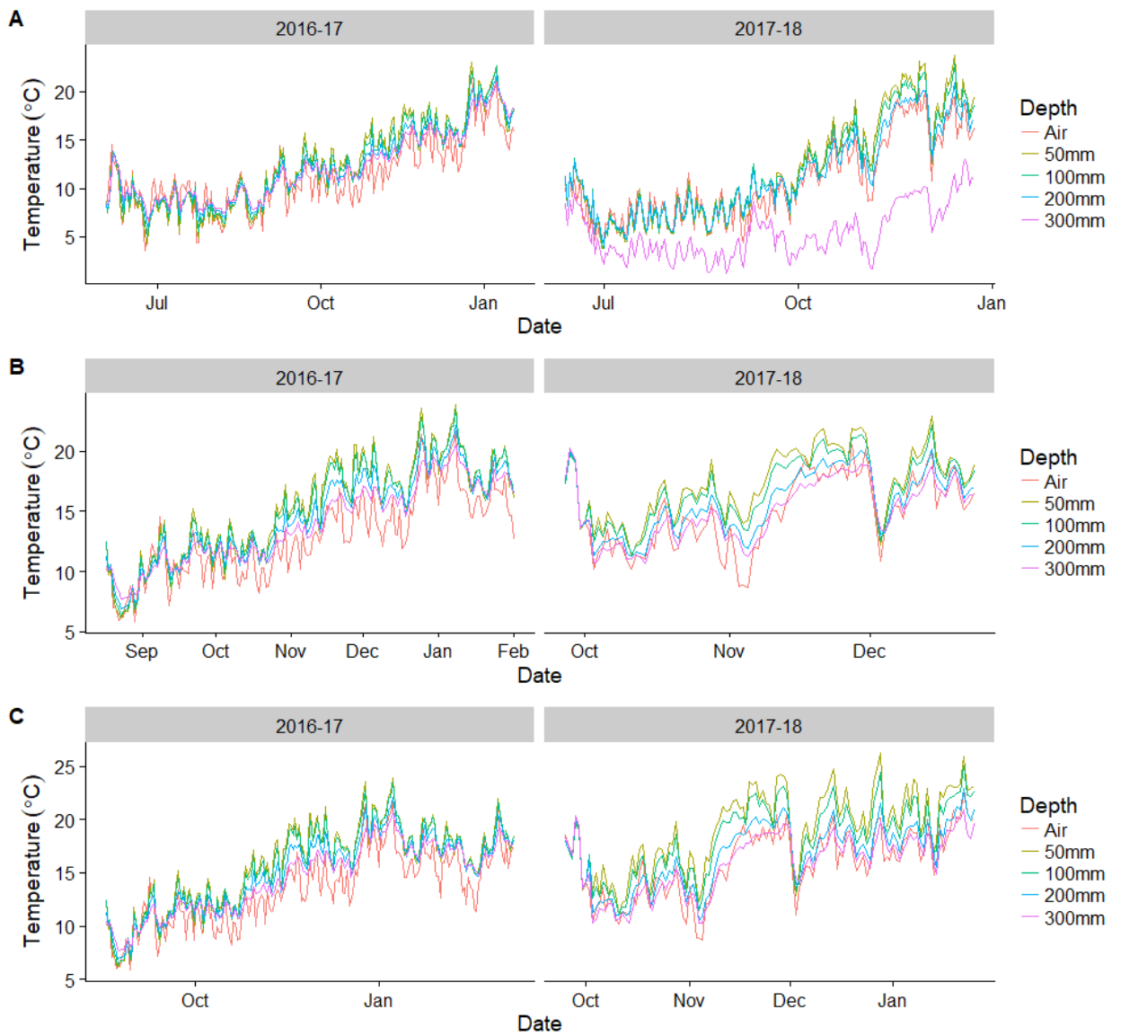
Figure 9. Temperature plots from planter bag trials showing mean daily temperatures of soil at varying depths in the profile as well as ambient air temperature. Planting windows are indicated as: A = Early, B= Intermediate and C = Late. Loggers were located at a single site and in close proximity. Logger data for the Early planting (A) in 2017-18 was used for the period from early August to late September.
