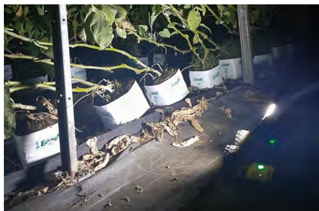
Image 3: The robot was designed to operate at night and used artificial lighting to illuminate the eggplant fruit.
