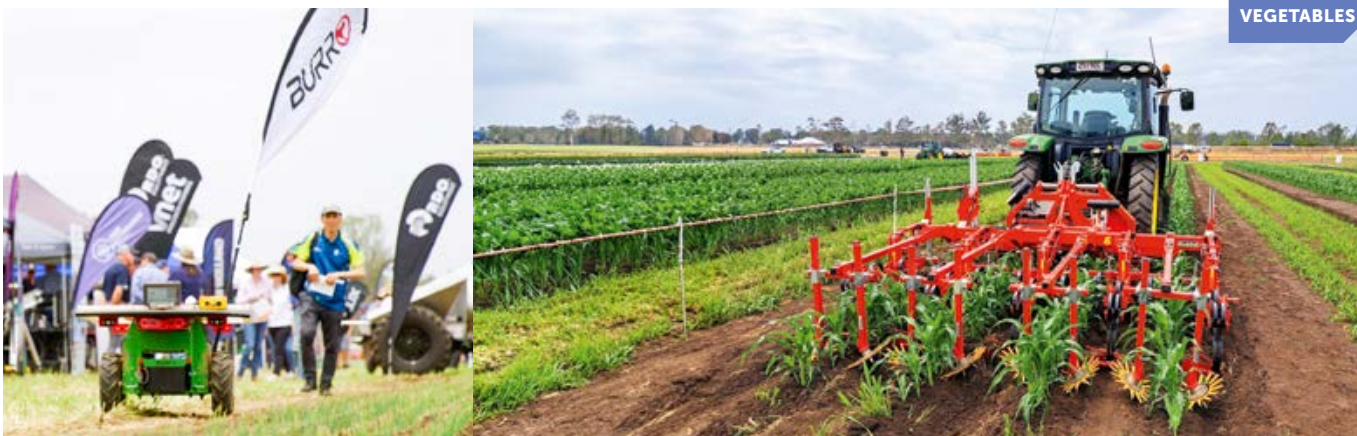
Above L-R. Autonomous agtech was on display at the Gatton Smart Farm AgTech Showcase in November 2023. Einbock row guard precision guided cultivator: precision inter-row weeder, Gatton Smart Farm AgTech Showcase.
