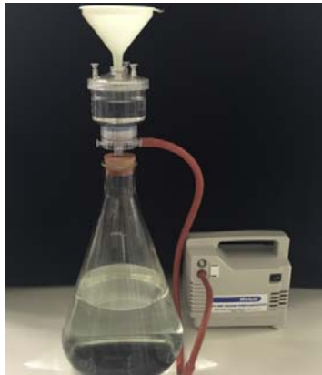
Figure 8: Millipore filter set-up for detecting bacterial cells.
