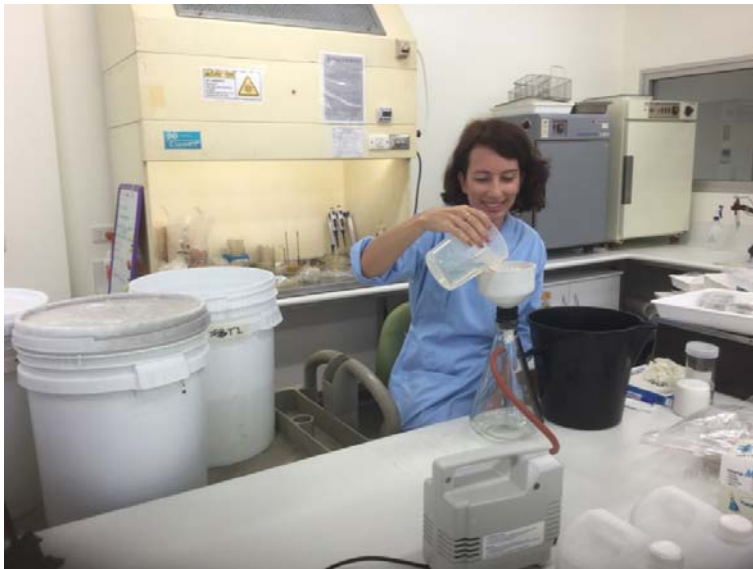
Figure 14: Technician pouring filtered water into Büchner funnel with Whatman No 42 filter paper used for fungal and oomycete detection.
