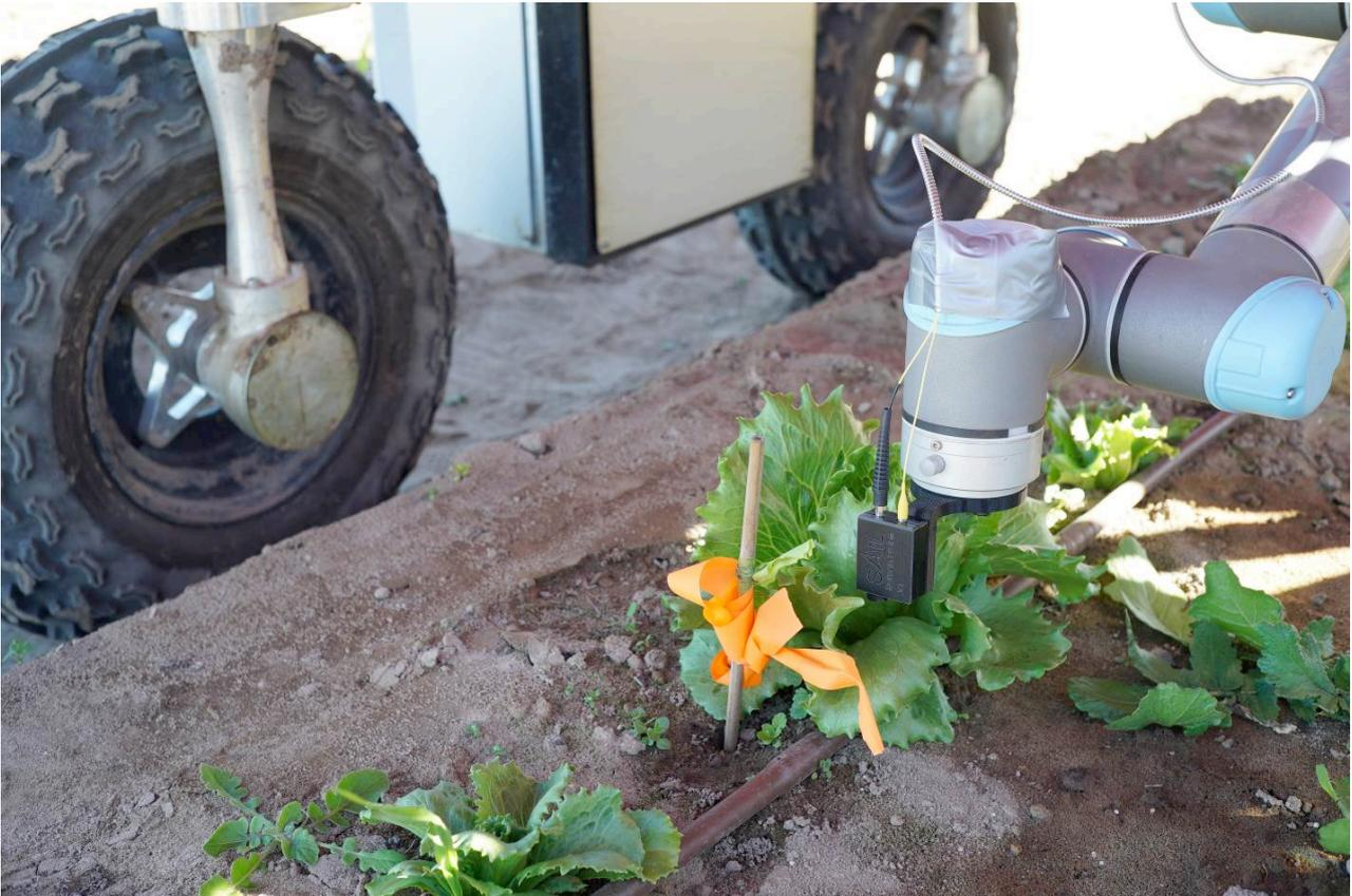
*Figure 12 – Raman sensor probe being positioned above the lettuce leaf.*
