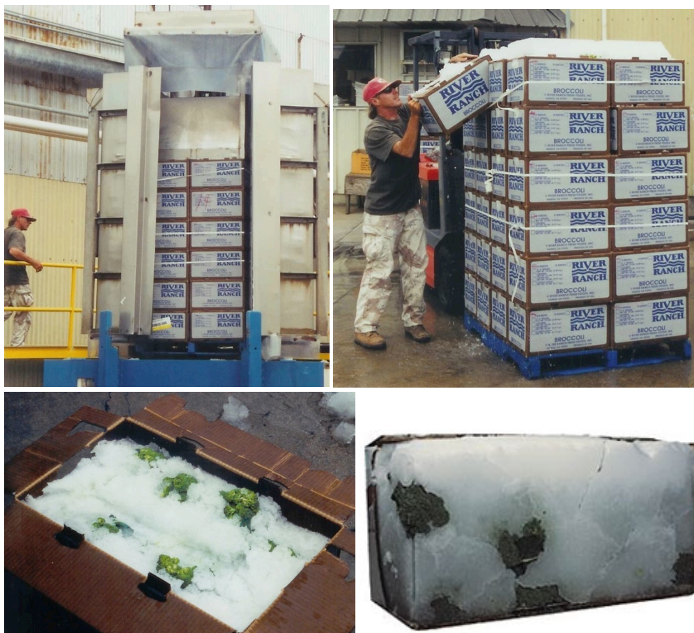
Figure 2. Broccoli icing in California using an ice slurry injection system (top). The result is a carton entirely filled with crushed ice and broccoli (bottom).
