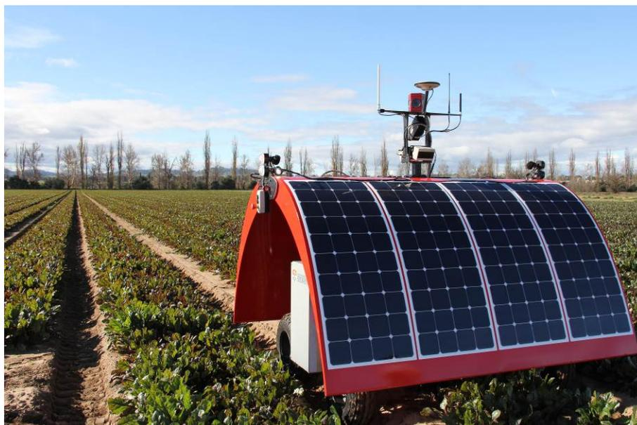
**Fig.2.** 'Ladybird' proof-of-concept robotic platform for use in vegetables
