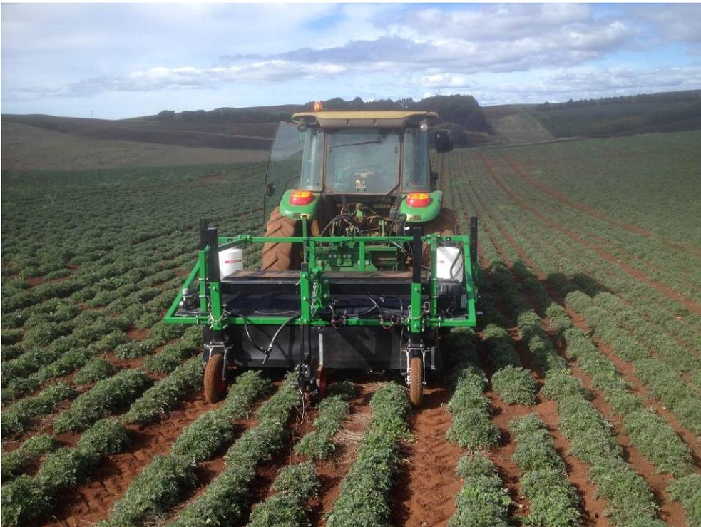
**Fig. 3.** Field test unit of selective weed sprayer being used in pyrethrum
