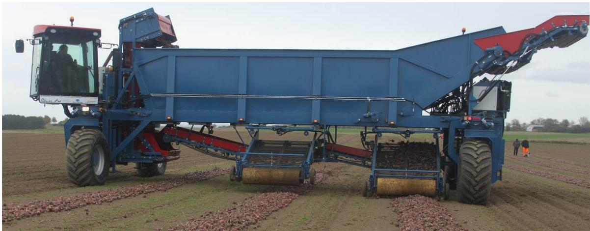
**Fig. 4.** Prototype wide-span gantry tractor developed by ASA-Lift, configured for onion harvest.
